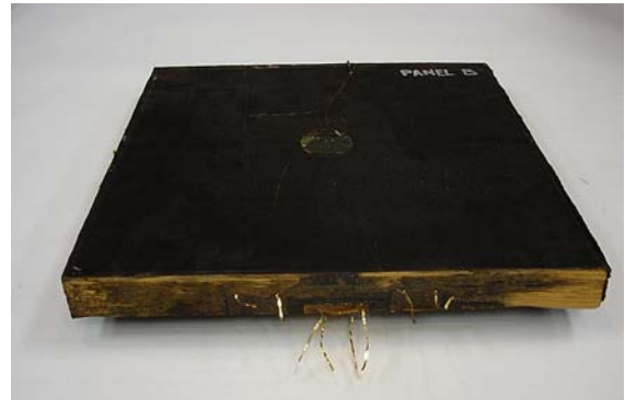
Fig. 6 A photograph of the thick 192 ply epoxy laminate with the embedded sensors after cure
